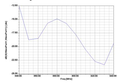
Figure 11. The input port-1 Scattering-parameters of this antenna
