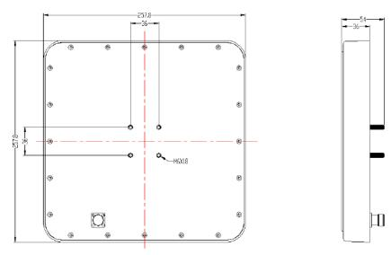
Figure 2 Dimension of the antenna
