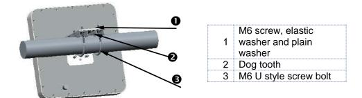
Figure 4. The structure for the Step 2 in the first case
