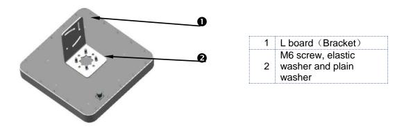
Figure 3 The structure for the Step 1 in the first case
