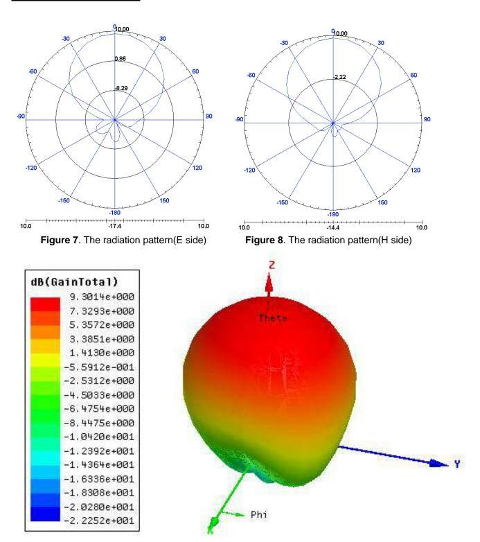
Figure 9. The radiation pattern(3D pattern, Gain> 9 dBi)
