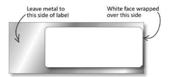
Smallest recommended bending diameter of the Confidex Flex™ is 50mm. For optimal read range please bend the label in the orientation shown below. Note that with smaller assets it is recommended to bend the label to other direction for optimal adhesion.
